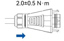
Figure 4.9. Tightening the nut
