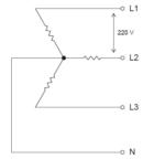
Figure 4.5. Connecting to three-phase power grid
