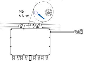
Figure 3.5. Installing the grounding cable
