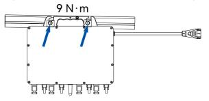
Figure 3.4. Mounting the microinverter
