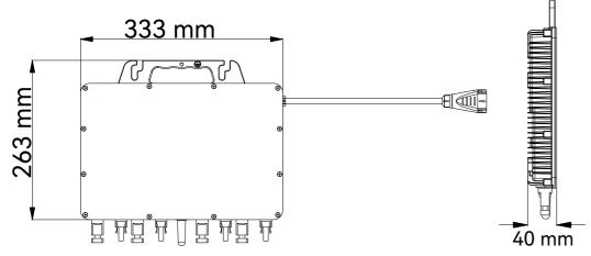
Figure 2.2. Dimensions of M2 microinverter
