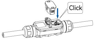
Figure 4.18. Inserting the port cap
