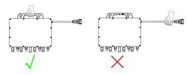
Figure 3.1. Carrying the microinverter
