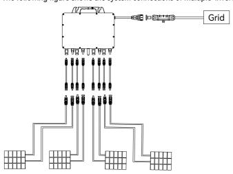
Figure 4.2. Multiple-inverter system connections
