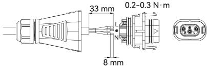
Figure 4.7. Crimping and inserting the cables
