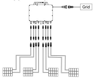
Figure 4.1. Single-inverter system connections
