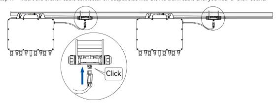
Figure 4.17. Connecting the AC cable
