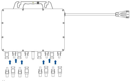
Figure 4.23. Connecting the DC cables
