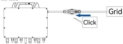
Figure 4.10. Connecting the AC cable
