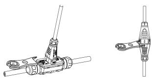
Figure 4.19. Disconnecting the AC connector
