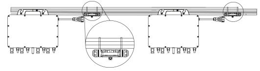
Figure 4.16. Laying the AC cables
