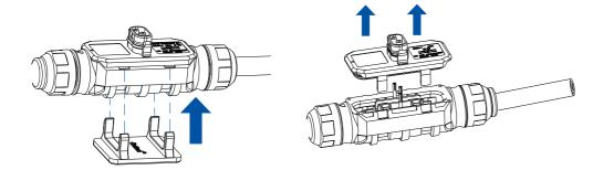
Figure 4.11. Removing the front lid
